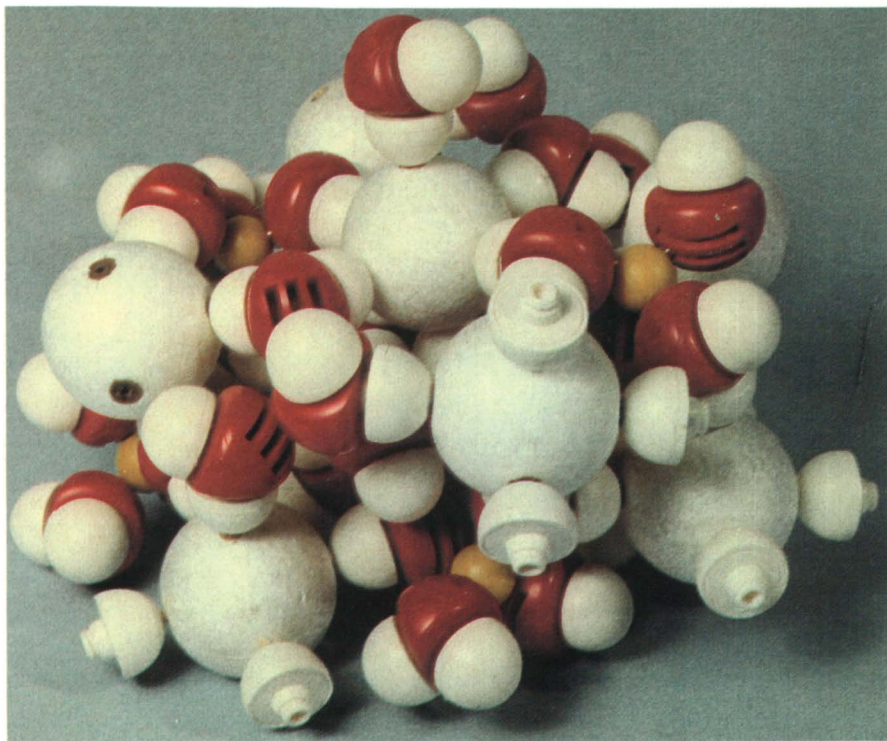
COLOR PLATE 16. Molecular model of \text{Li}^+(\text{nH}_2\text{O})\text{Cl}^- , water-bridged ion clusters in glasses at 100 K, derived from pulsed ^1\text{H} NMR data.
